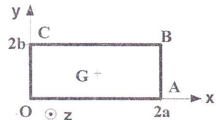
$$\vec{V}(B/R) = \left[ \frac{d}{dt} \overline{OB} \right]_R = \left[ \frac{d}{dt} \overline{OA} \right]_R + \left[ \frac{d}{dt} \overline{AB} \right]_R = a \left[ \frac{d}{dt} \vec{x}_1 \right]_R + b \left[ \frac{d}{dt} \vec{x}_2 \right]_R$$
